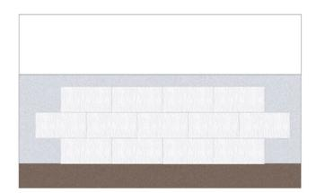
EPS Geofoam can be used as a compensating foundation to reduce the load on underlying compressible soils and minimize building settlement along with potential bearing capacity problems. Existing soil is excavated to reduce the net applied load to the soil by the new structure. If the amount of soil excavated equals the full weight or stress applied by the new structure, the foundation is called "floating" or "fully compensating."
