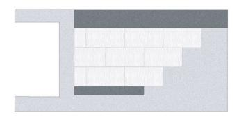
EPS Geofoam can be used to support bridges when designed to the proper specification. The material adds little additional load to the underlying ground and therefore is a perfect material for the construction of a bridge structure. In cases of a rehabilitation of a bridge which is no longer structurally stable to hold the loads of current traffic loads, EPS Geofoam infill can help support the span and transfer the traffic load safely to the foundation or underlying soil.
