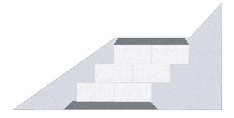
The use of EPS Geofoam on a side hill project is common practice and has been used for years. The reduction of weight and pressure against the side of the hill is used to prevent landslides, and stabilize the hill side. The lack of increased weight on the side of the hill allows for a safer, more stable road construction project. As a rule of thumb, Geofoam is up to 1000 times lighter than other traditional fills with similar compressive strengths.
