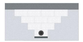
A great use for EPS Geofoam is the covering and protecting of underground utilities. The EPS distributes weight evenly around the piping or utility lines and reduces the amount of pressure and force on the ground. It reduces the vertical stress on pipes and other sensitive utilities. This reduction in weight on top of the utility lines will prevent potential issues like collapses.
