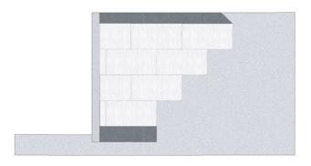
Using a EPS Geofoam product in a retaining structure will provide less lateral pressure and prevent any settlement. It is also good for improving water-proofing as the EPS Geofoam is a closed cell material and will not rot, leach into the ground, or decompose over time. The light weight aspects of the material reduce lateral force on a retaining wall or abutment. Most teams will install a draining system below the geofoam to prevent any hydrostatic pressure or buoyancy.
